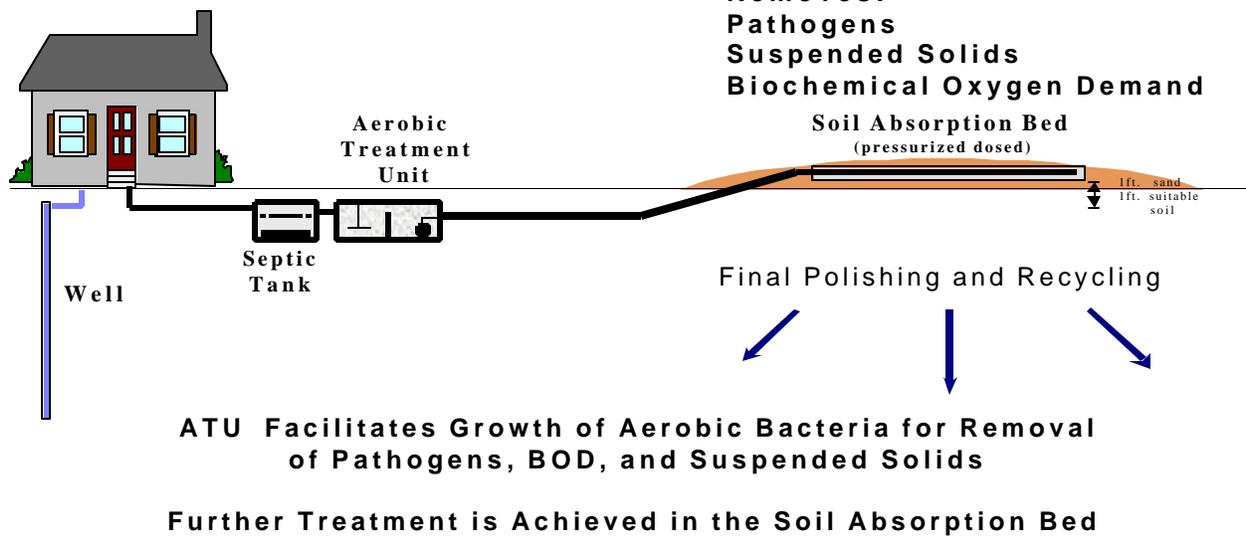
An Aerobic Treatment Unit (ATU) is a self-contained unit that uses blowers or propellers to aerate the wastewater. They may also have filters to remove suspended solids. The additional electrical components are no more complicated than those commonly used in mound systems. An onsite sewage system that incorporates an ATU has either a septic tank or contains a septic compartment for solids separation, followed by the ATU, and a soil absorption bed.
