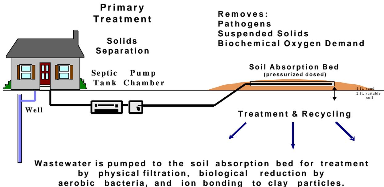
A mound system, like a conventional system, consists of a septic tank and a soil absorption bed. In the mound system, however, sand is added where suitable native soil is insufficient. Clarified effluent from the septic tank is pumped, in controlled pressurized doses, to an aboveground, free-standing sand layer. The sand layer, placed upon a specially prepared area of native soil, serves as the medium on which aerobic bacteria facilitate much of the secondary treatment.
