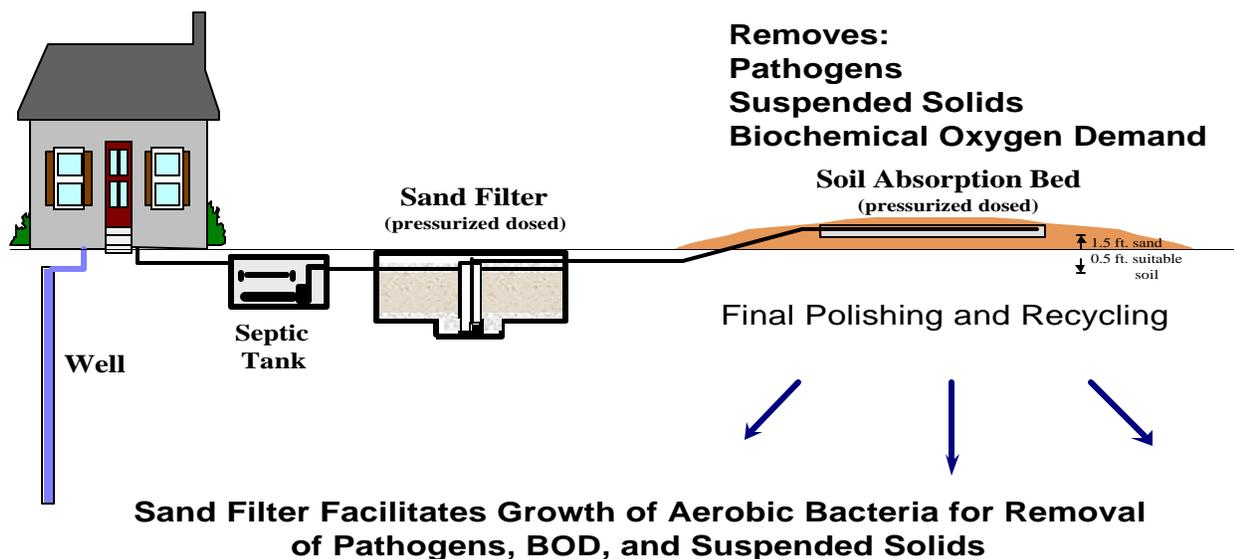
**Sand Filter Facilitates Growth of Aerobic Bacteria for Removal of Pathogens, BOD, and Suspended Solids**
