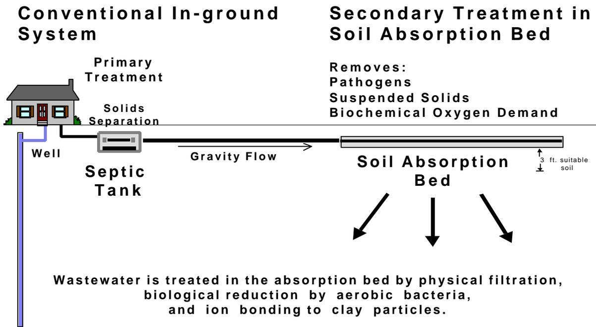
A conventional in-ground septic system consists of a septic tank and a subsurface soil absorption bed. In the septic tank, solids settle out of the waste stream and anaerobic bacteria facilitate the partial breakdown of organic matter (primary treatment). Clarified effluent from the septic tank discharges via gravity to a soil absorption bed.
