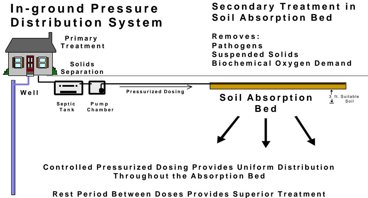
An in-ground pressure distribution system consists of a septic tank, pump chamber, and a sub-surface soil absorption bed. Including space for the drain tile, gravel trench and overlying fill, the minimum native soil requirements range from 49 to 53 inches depending on the diameter of the distribution pipes. Like a conventional system, 36 inches of suitable native soil above bedrock or groundwater is required for the absorption bed.
